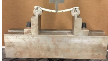
Figure 3: Flexure Testing Apparatus, Specimen Supports and Loading Nose for Three-Point Bending During a Three-Point Bending Test of a M13 Specimen
