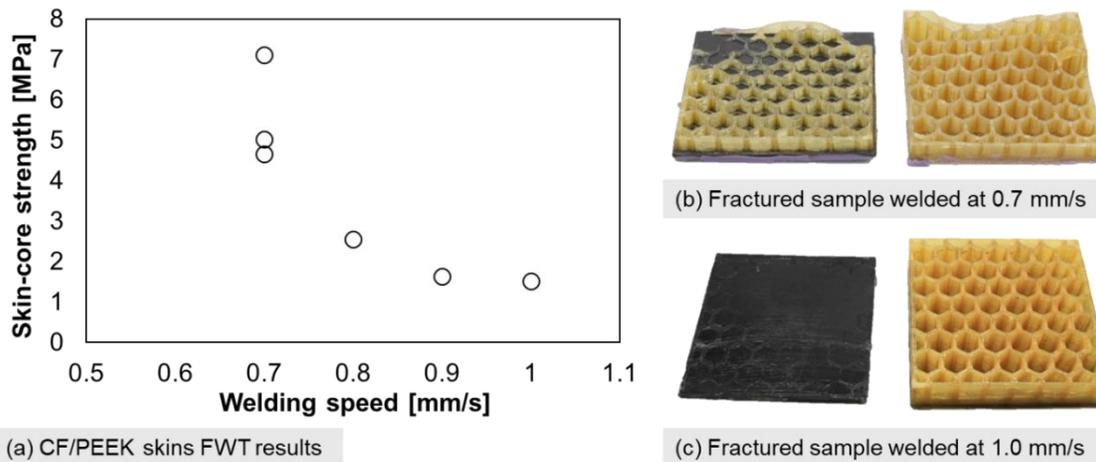
Figure 4. (a) CF/PEEK FWT test results. Fractured samples welded at (b) 0.7 mm/s and (c) 1.0 mm/s are presented.
