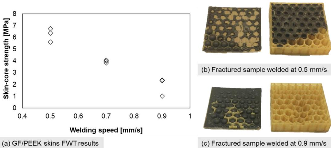
Figure 3. (a) GF/PEEK FWT test results. Fractured samples welded at (b) 0.5 mm/s and (c) 0.9 mm/s are presented.
