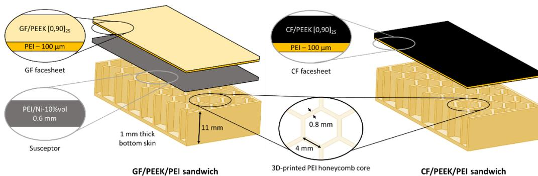
Figure 1. Schematics of GF/PEEK/PEI and CF/PEEK/PEI sandwich samples.
