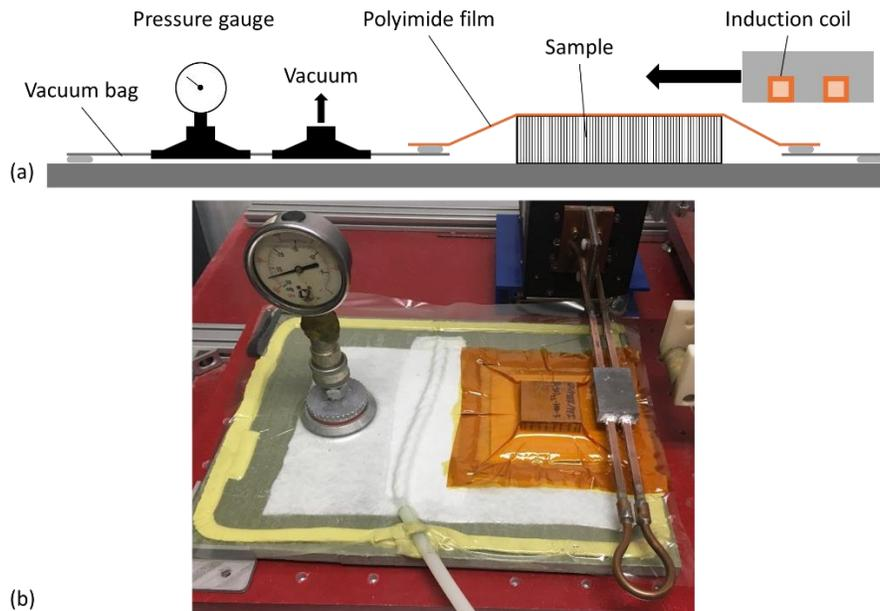
Figure 2. (a) Schematic and (b) picture of the vacuum assisted induction welding (Vac-IW) setup. Reproduced from [14].
