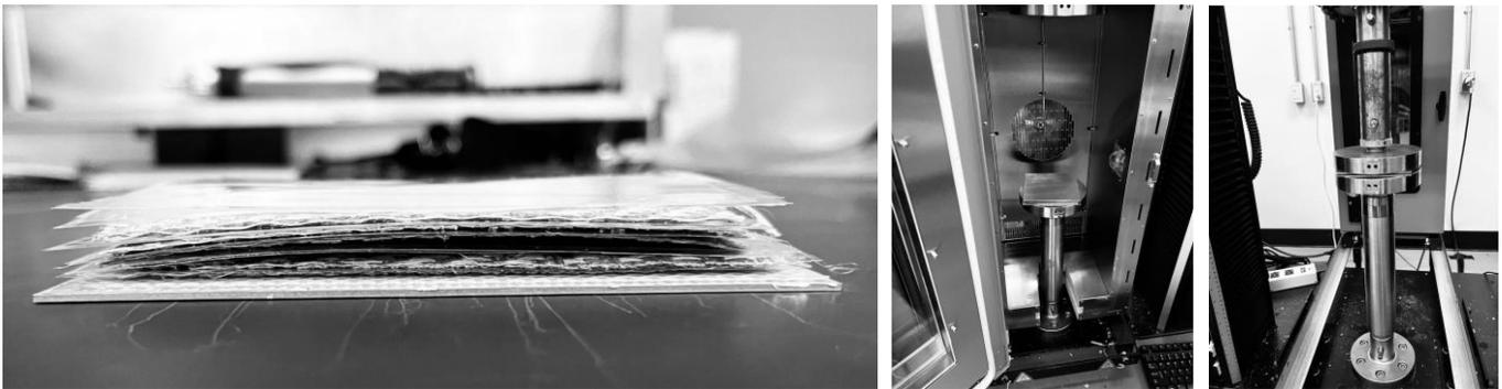
Figure 2. Hot compression lamination. Left: stack with top silicone and metal sheets removed for clarity; centre: stack on lower platen in Instron oven; right: stack compressed between platens with oven rolled back for clarity.
