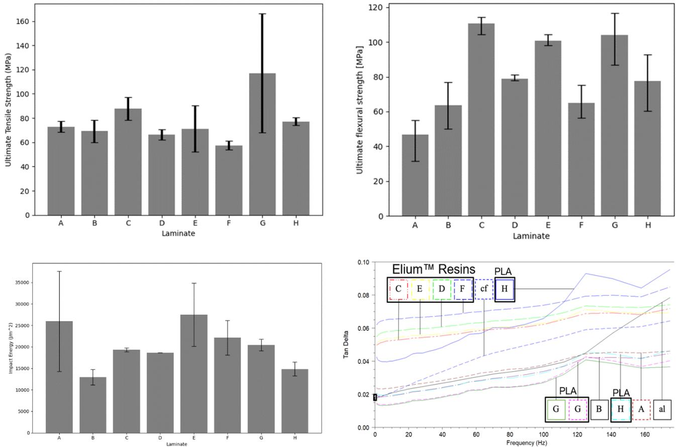
Figure 4. Select composites characterization results. Top left: tensile strength; top right: flexural strength; lower left: impact strength; lower right: DMA results. A – Resin #1 & Fabric #1; B – Resin #1 & Fabric #2; C – Resin #2 & Fabric #1; D – Resin #2 & Fabric #2; E – Resin #3 & Fabric #1; F – Resin #3 & Fabric #2; G – Resin #4 & Fabric #1; H – Resin #4 & Fabric #2.
