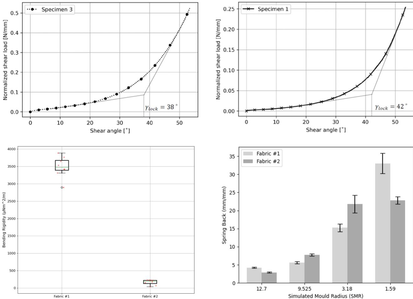
Figure 3. Select dry fabrics characterization results. Top left: in-plane shear curve, Fabric #1; top-right, in-plane shear curve, Fabric #2; lower left: bending stiffness, both fabrics; lower right: spring back ratio, both fabrics.
