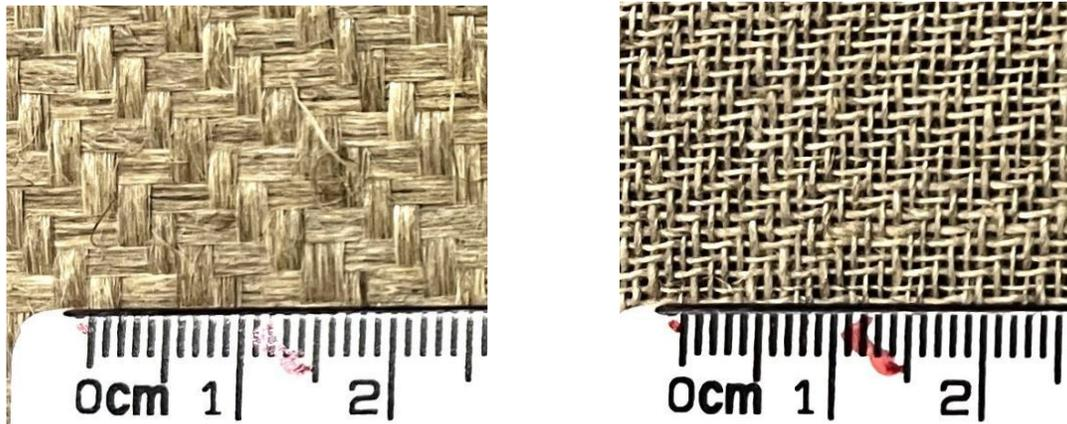
Figure 1. Flax fibre reinforcement fabrics. Left: TEXONIC TF-05-T; right: EcoTechnilin FLAXDRY BL200.
