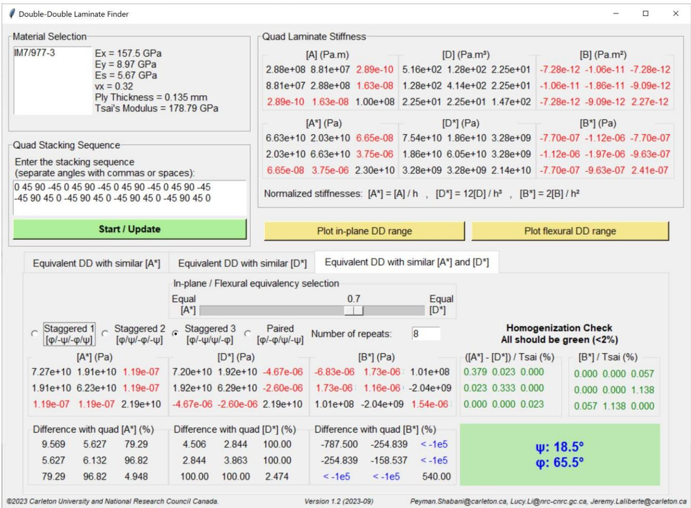
Figure 1. Developed tool for finding equivalent Double-Double laminates.
