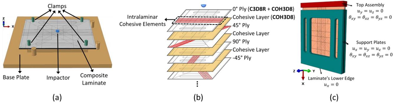
Figure 2. (a) FE model assembly for LVI simulation, (b) Embedded cohesive elements inside laminate, (c) FE model assembly and boundary conditions for CAI simulation.
