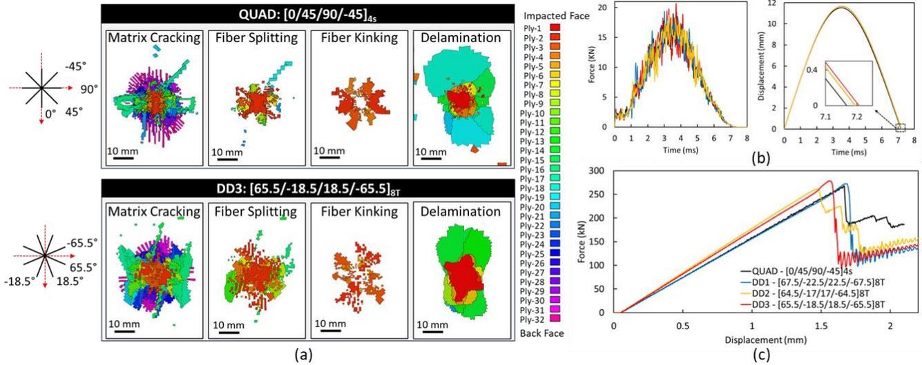
Figure 3. (a) Inter- and intra-laminar failure modes predicted for QUAD and the chosen DD laminate after a 75 J impact event, (b) LVI responses of QUAD and DD laminates, (c) CAI force-displacement diagrams.
