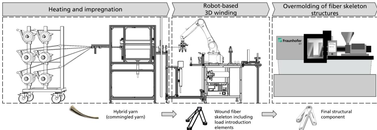
Figure 1. Process chain of the 3DSW process [2]
