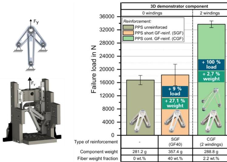
Figure 3. Failure loads in tensile direction of the generic 3D demonstrator component [2]
