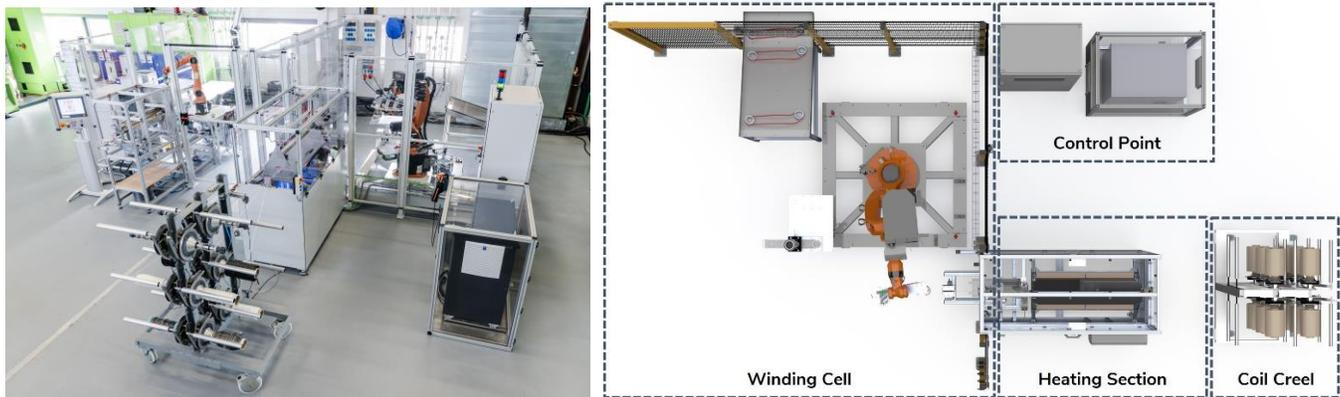
Figure 2. Industrialized 3DSW production line developed by Fraunhofer ICT and Fritz Automation GmbH (left); Illustration of the 3DSW units (right)
