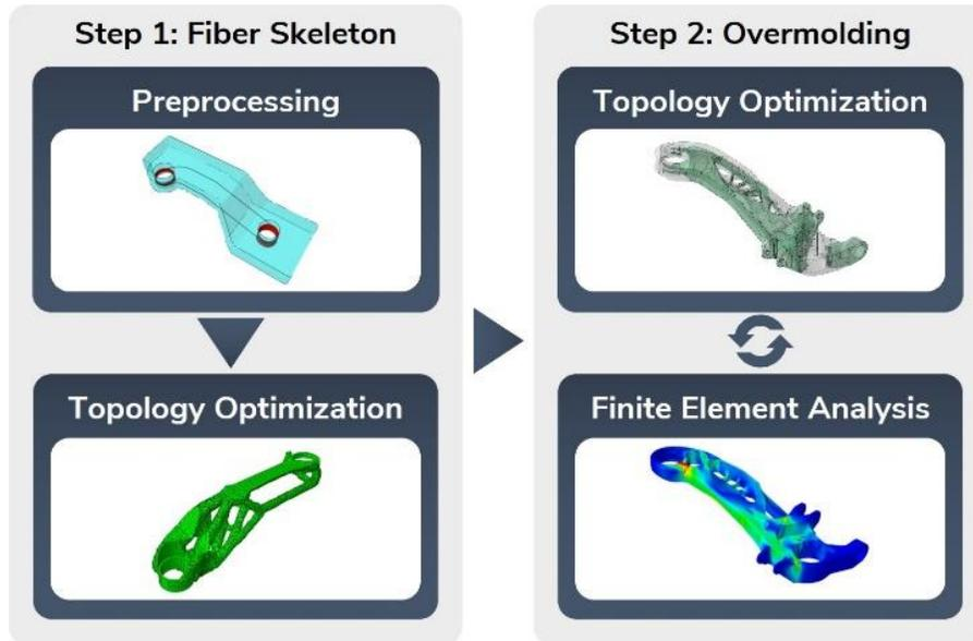
Figure 4. Schematic illustration of the algorithmic virtual optimization and validation approach for 3DSW structures
