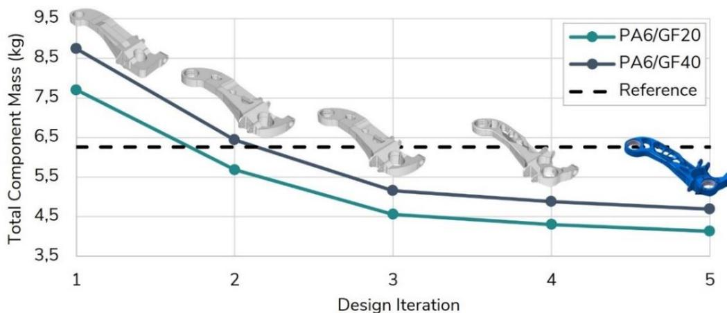
Figure 5. Evolution of component mass along with the design iterations and comparison to the metallic reference component
