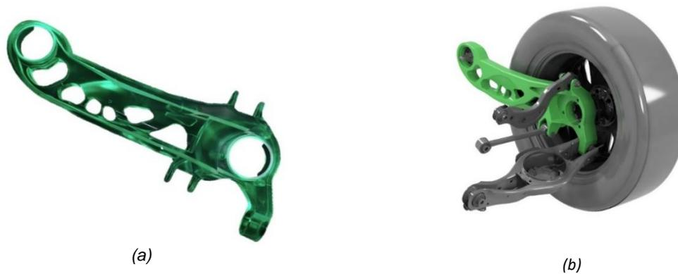
Figure 6. 3DSW rear trailing arm demonstrator: Photograph of the demonstrator (a) and CAD assembly (b).
