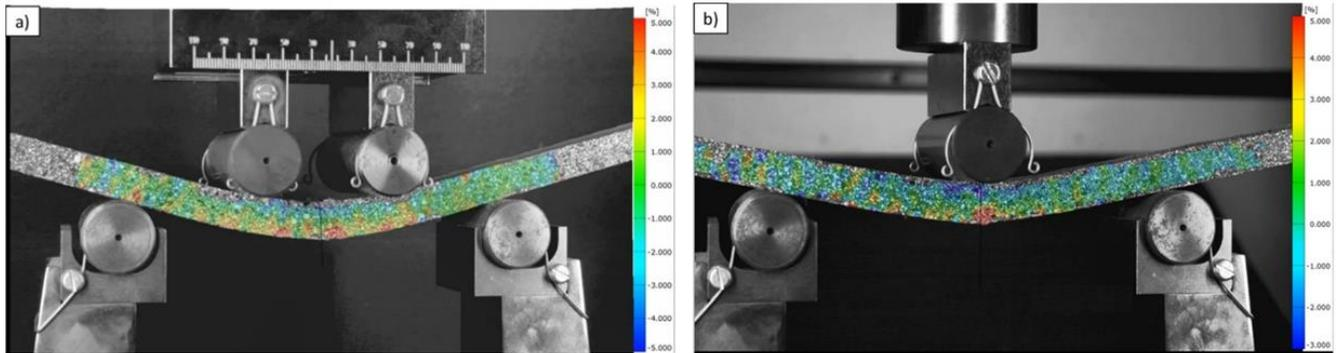
Figure 3. a) Full-field strain of composite specimen under four-point bending test just before failure, b) Full-field strain of composite specimen under three-point bending test just before failure.
