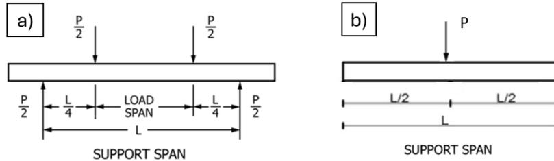
Figure 1. a) Four-point bending test diagram, b) Three-point bending test diagram (ASTM D6272) [5][6].
