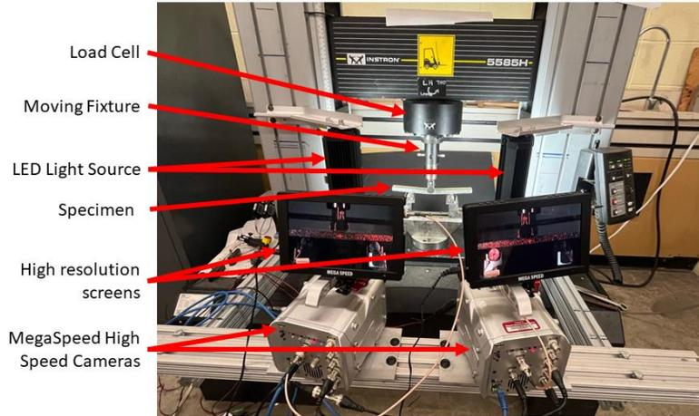
Figure 2. Instron 5585H load frame with high-speed stereo system for 3D digital image correlation (3D-DIC) test setup.
