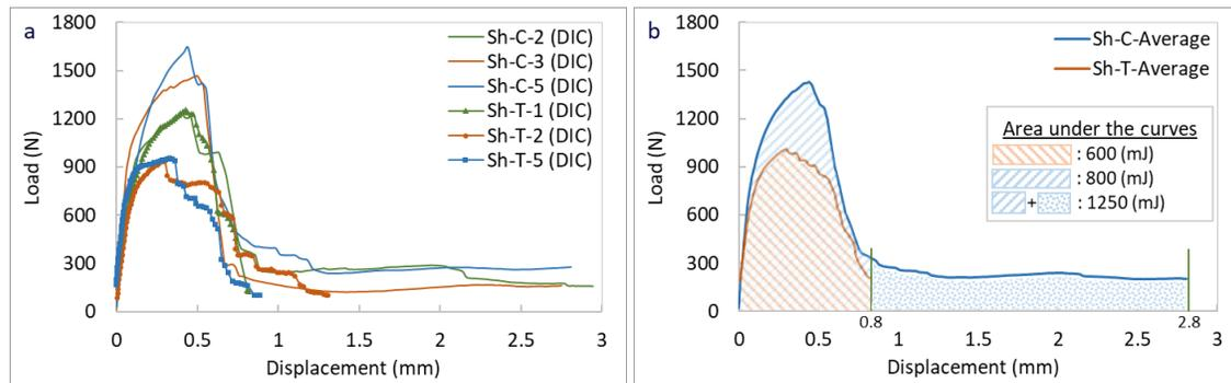
Figure 3. Load-displacement diagrams for a) Both test configurations, b) Average of each test configuration, with corresponding dissipated energy.
