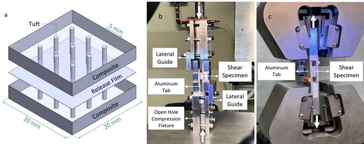
Figure 1. a) Schematic of shear specimen. b) Compression loading setup with lateral guides. c) Tensile loading setup.
