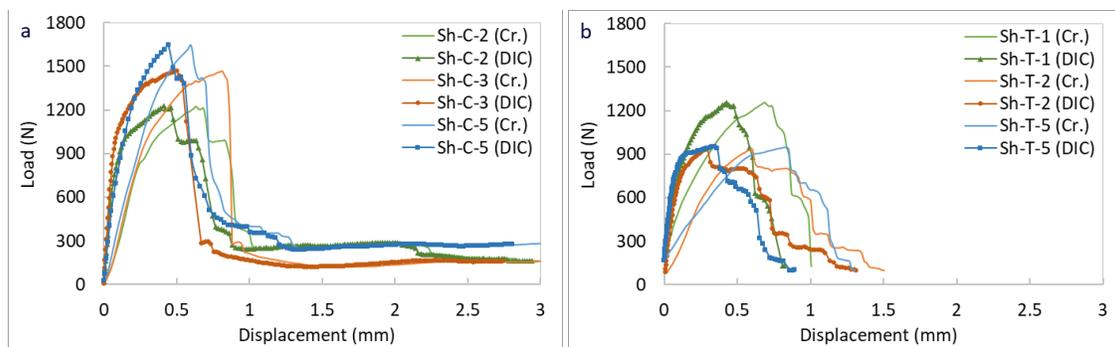
Figure 2. Load-displacement diagrams from Crosshead (Cr.) and DIC measurements for a) Compression test setup with the lateral support, b) Tensile test setup.
