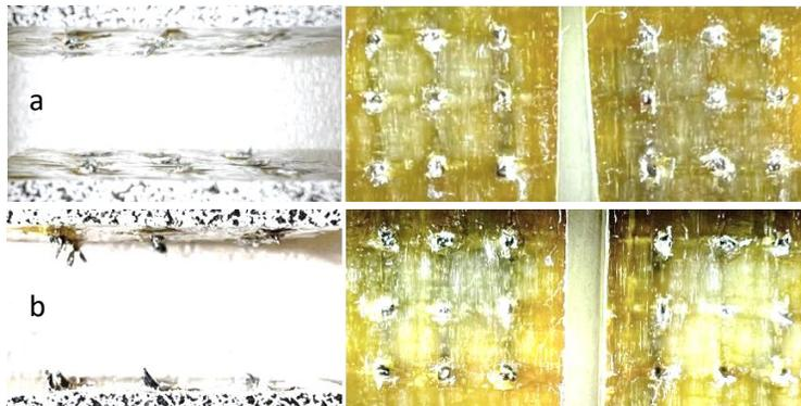
Figure 5. Fracture surface of the specimen tested by a) Compression test setup with lateral guides, b) Tensile test setup.
