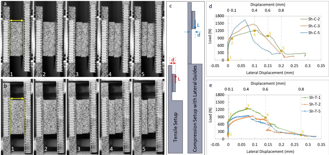
Figure 4. Lateral displacement during the test in a) Compression setup with lateral guides, b) Tensile setup. c) Schematic of load and resulting bending moment in half of the tensile and compression tab/specimen assembly. Load-lateral displacement diagrams for d) Compression setup with lateral guides, e) Tensile setup.
